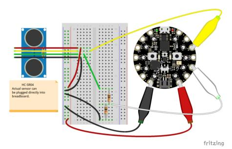
The picture below shows how it looks implemented on a breadboard. The only differ ences are: the sensor is plugged into the breadboard; the use of double-ended alligator (crocodile) clip leads with header pins aiding connection to the breadboard. The alligator clip to male jumper wire (https://adafru.it/CuB) is an easier alternative.
