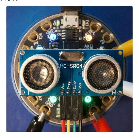
The HC-SR04 is an inexpensive distance sensor based on a pair of <a href="ultrasonic transducers"><u>ultrasonic transducers</u></a> (https://adafru.it/CxB) with a straightforward <a href="TTL"><u>TTL</u></a> (https://adafru.it/CxC) level interface and a claimed range of 2cm to 4m. Similar sensors are now commonplace with the widespread use of car parking assistance sensors.
