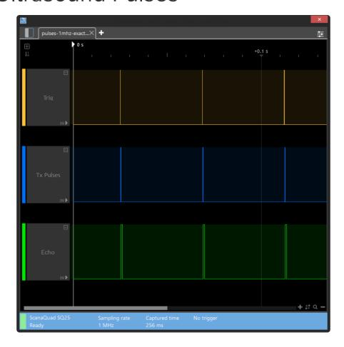
A logic analyser can be used to look at the communication between the CPX board and sensor. It can also be connected to the ultrasonic transmitter to see the high frequency chirp but won't work on the unamplified receiver output. A basic logic analyser cannot show the full detail of the analogue voltages as it makes everything appear rectangular. There are some examples of what the signal really looks like on  $\underline{D}$  avid Pilling's HC-SR04 page (https://adafru.it/CxI).
