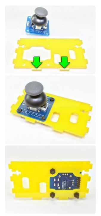
When installing the joystick on this support piece, make sure these two bumps are at the bottom.
