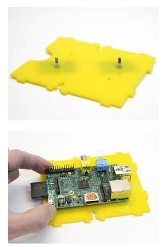
Set the piece down on your work surface with the screws pointing up, then add a nylon spacer over each screw.
