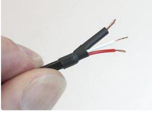
Strip 1/4" insulation from the two inner wires. Twist the stranded copper wire into a tidy bundle.
