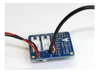
The speaker and headphone wires then connect to corresponding points on the board. The speaker wires go to the two "Spkr" points, headphone to the three "Audio" points: red wire to "R," black or white wire to "L," copper wire to "GND."
