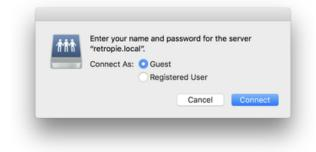
Here's how one typically connects from a Mac, using the Finder's Go→Connect to Server... option. Windows, Linux will have their own equivalent functions.
