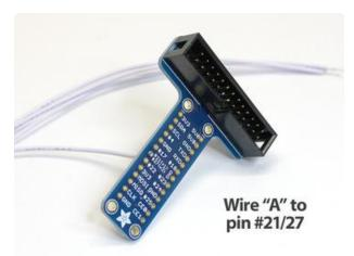
Using the schematic at the top of this page for reference, solder the other end of the wire to the appropriate point on the T-Cobbler. Wire A goes to Pin #21/27
