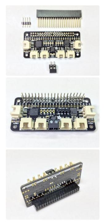
Three components are soldered to the Arcade Bonnet board:
