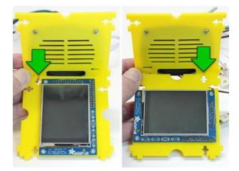
The screen fits into two slots at the bottom of the speaker grille.
