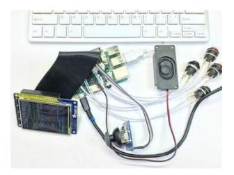
Spread out the parts on your work surface, making sure no metal bits contact each other. Connect a USB keyboard and then connect power to the Pi.
