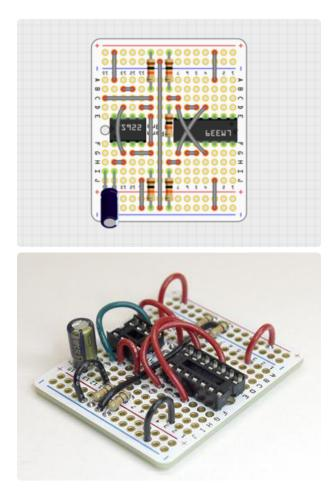
Install the 100  $\mu$ F capacitor in the position shown.
