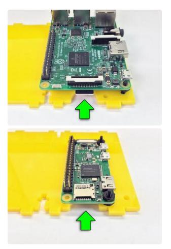
Now set the Raspberry Pi atop the screws. Only three of the board's four mounting holes are used (the fourth would interfere with other parts of the case).
