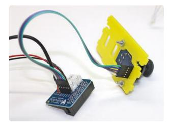
Connect the female jumper wires between the joystick and Cupcade board, making sure you get the same sequence (e.g. GND to GND and so forth). If you get these out of sequence, the Pi might not boot!
