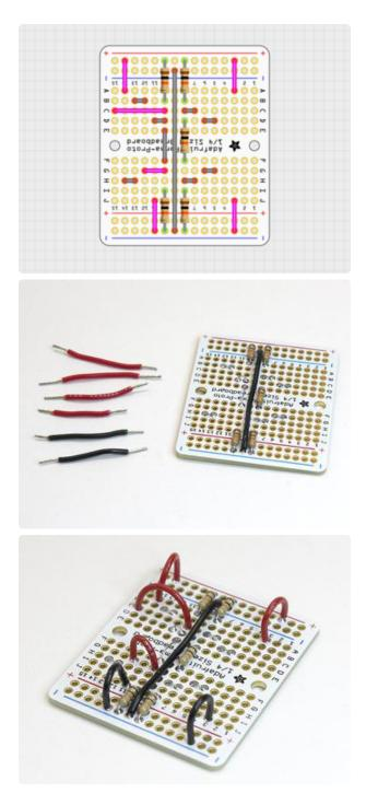
Six more jumpers are now installed as shown in pink (prior steps are gray). Because these jumpers cross other traces, they should be cut from insulated wire, <u>do not</u> use the resistor clippings for this step!
