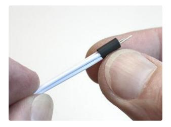
Gather up four quick-connects (the unlabeled ones) and squeeze the tips through a piece of heat-shrink tube.
