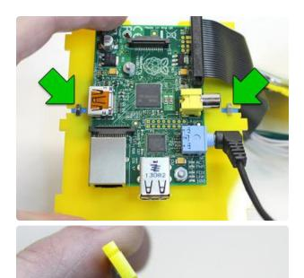
Then, from the top side, press a nut into the cross part of each "T." Give it a pinch from both sides, so the tape gets a good hold on the nut.
