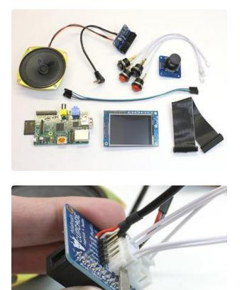
With the Pi powered off, disconnect all of the separable parts:
