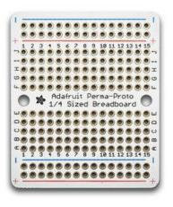
Generation 1 kits had you solder up several components and wires on an Adafruit Perma Proto board.
