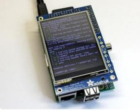
amiss with the PiTFT assembly. Is it plugged in right? (Sometimes the header pins are off-by-one and it doesn't work.)
