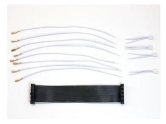
Clip the 2-pin plastic plugs off the button quick-connects. You should then have eight (8) wires with a metal spade on one end. Strip a little insulation from the other end.
