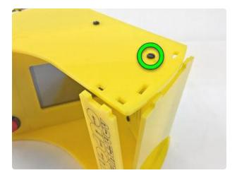
Loosen this screw to insert the cabinet marquee and "roof" piece, then retighten.
