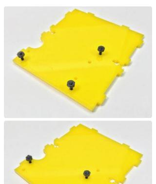
Insert a screw, coming up from the underside, through each of the three mounting holes...whichever set you're using...then add a nut from the top side.
