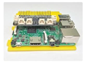
Install the Arcade Bonnet atop the Pi GPIO header as you did during the dry run.
