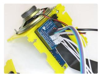
The Cupcade board plugs into the back of the PiTFT as it was during our dry run.
