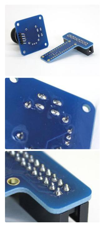
Make sure all your solder connections are smooth and clean, like tiny Hershey's Kisses<sup>®</sup>. There should be no solder balls or bridges, no gaps between pins and their corresponding pads.
