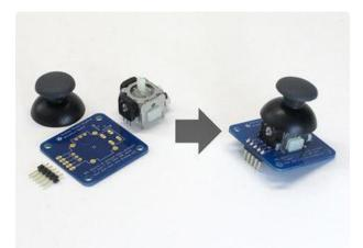
The analog thumb joystick board has a 5pin header and quite a few pins on the stick component itself. Some of the pins may be a little bent from shipping and need to be nudged into place. The "hat" simply presses into place.
