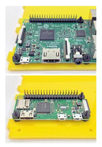
Here's how it looks when properly installed. Nuts are flush with both sides of the board, not pinching down on components. And the board is elevated at just the right height for the SD card slot and side cutouts to work.
