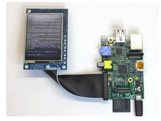
Turn the screen over and connect a USB keyboard and power. After a few seconds you should see the same bootup sequence as before. If the PiTFT worked when connected directly to the Pi but does not work with the ribbon cable:
