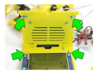
Add tape behind the two T-slots at the top of the speaker grille, then press nuts into place.
