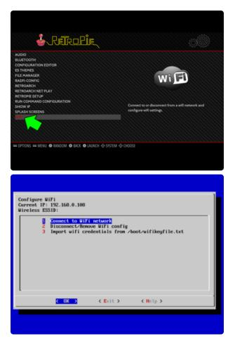
Highlight the "WiFi" option at the bottom of this list and press the A button again. This runs a WiFi configuration utility, which is all text-based...so this works with the keyboard's arrow keys, tab and enter keys to select menu items, and when asked for the network password just use the keyboard as normal.
