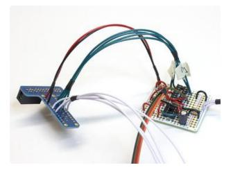
The four direction wires (U, D, L, R) can now be soldered to the appropriate positions on the Perma-Proto board. Refer to the schematic.
