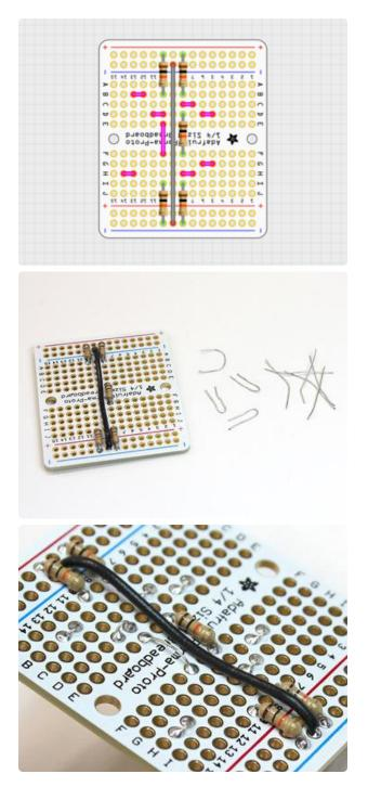
Eight short jumpers are now installed in the positions shown in pink. Most of these are very small, joining adjacent pads. We can use the un-insulated clippings from the prior step because no other conductive traces are crossed.
