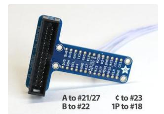
Repeat with the other three wires, <u>one at</u> <u>a time</u> so you don't get them mixed up. Slide one wire part way out of the heatshrink, grab the "tail" and solder in to the correct spot:
