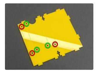
The base piece has board outlines scored on the top surface, and six mounting holes. The three "inner" holes (outlined in green) are for Raspberry Pi Zero boards, while the "outer" holes (outlined red) are for a Pi 3, Pi 2, etc. We'll use just one set or the other, depending which board you've got.
