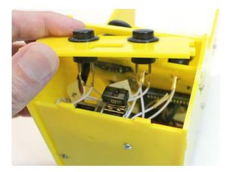
Friendly reminder: this is your last chance to add a USB mini WiFi adapter if you want! Plug it into the top USB slot. Leave the bottom slot open for a keyboard.
