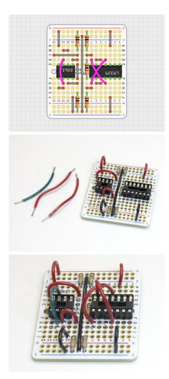
Three more jumpers are installed, cut from insulated wire.
