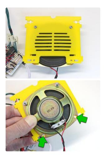
Install the speaker grille using two screws at the top.
