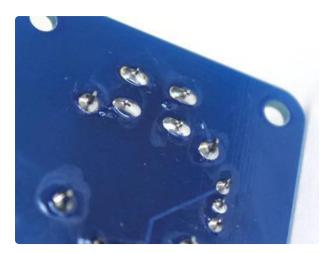
Make sure all your solder connections are smooth and clean, like tiny Hershey's Kisses<sup>®</sup>. There should be no solder balls or bridges, no gaps between pins and their corresponding pads.
