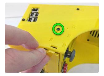
Loosen a screw and lift up the case side to install this front piece just below the joystick and buttons. There should be just enough clearance and flex for this to happen. Bend too far and you'll crack plastic or pop the head off a screw.
