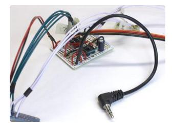
Solder the three wires to the proscribed locations on the Perma-Proto circuit.
