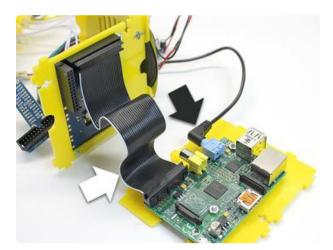
Plug the audio cable into the headphone jack and the ribbon cable to the GPIO header, making sure pin 1 (the white wire) is in the correct place.
