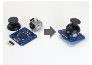
Assemble the analog thumb joystick. Some of the pins may be a little bent from shipping and need to be nudged into place. The "hat" simply presses into place.
