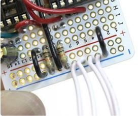
Solder the other end of these four wires to the lower ground bus on the Perma Proto board. The wires enter from the top and are soldered on the underside. Clip any excess wire protruding from the bottom.
