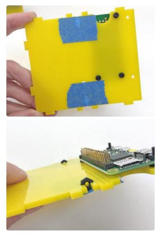
If using a Pi Zero, the sequence is a little different. Apply the tape first to the bottom face of the base piece, covering the two T-slots. Then, from above, slide a nut into each of the two slots. Really press them in to make sure they're making good contact with the tape.
