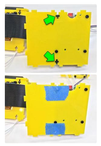
If using a Pi 3 or similar form-factor board, slide a nut into these two T-slots from the underside. The board with block them from slipping out the other side.
