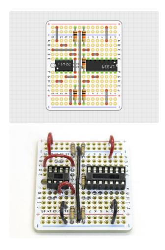
This diagram shows where the TS922 amplifier and LM339 comparator ICs will be installed later. In their place for now we'll install sockets, then add the chips after everything else is complete.
