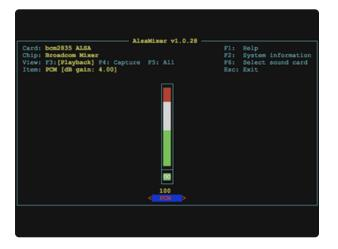
Press the up arrow until the volume level is at the maximum. Then press the Escape key to save and exit.
