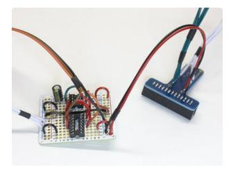
Solder the other end of the power wires to the appropriate positions on the Perma-Proto board, then heat-shrink the tubes near the ends.
