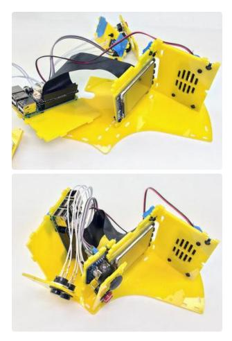
Take the jumble of parts and try to (roughly) align the tabs on the speaker grille, screen and joystick supports with the corresponding holes in the side piece. They probably won't stay in those holes for very long, but at least you'll know where they belong.
