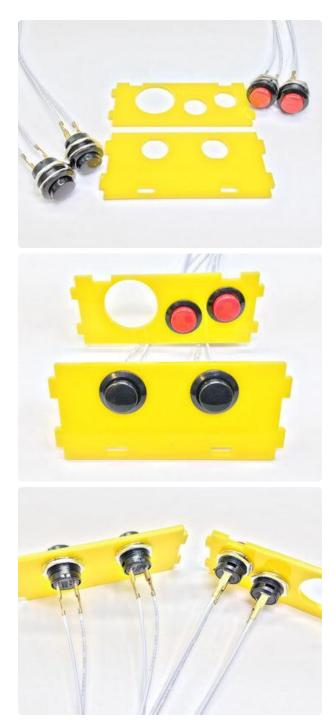
Insert the two red buttons into the chosen control cutout. The two black buttons then go in this cabinet front piece.
