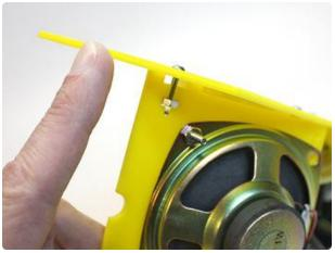
Loosen a side screw at the top. Same routine: screw tip flush with nut face, so you can flex this side up just a little bit.
