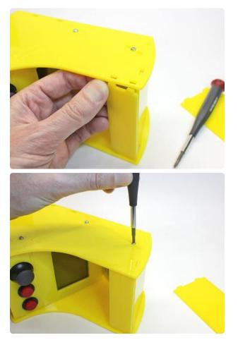
Slot the marquee into place, then retighten the top screw.
