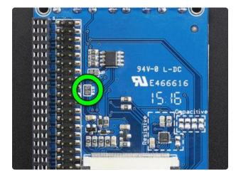
On the back of the PiTFT, near the GPIO pins, are two pads labeled "#18" with a narrow PCB trace between them.
