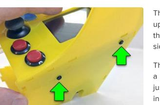
Fit the joystick and button supports into their own slots as you're working on this section. Use masking tape to hold these four pieces in alignment.
