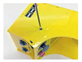
Here I'm starting with the joystick area... but you might want to start with the base piece instead; it has the fewest interferences. It's only because I've done this a few times and have the hang of it.
