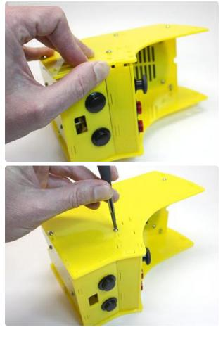
Install this fascia piece in a similar manner, then tighten the side screw back as it was.
