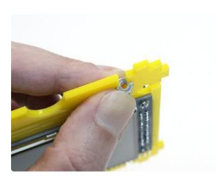
Bring the two pieces together and add a #4-40 1/2" screw. This will pass through the speaker frame, the plastic grille piece and into the nut.
