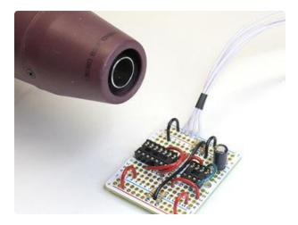
Now slide the heat-shrink back down the wires, about 3/4" from the board, and apply heat. Most people simply use a butane lighter for this, but if you have a heat gun that's even better.
