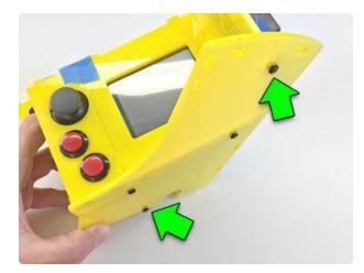
A third screw installs from the side at the top of the speaker grille piece.
