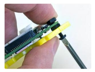
Instead, set a nut on the tip of one screw, and observe how it bumps up against nearby parts (such as the end of the GPIO header). You'll always find some orientation of the nut where it clears all the parts. Hold it in this orientation, then tighten the screw up from the bottom. The board will then be neatly sandwiched between the two nuts!
