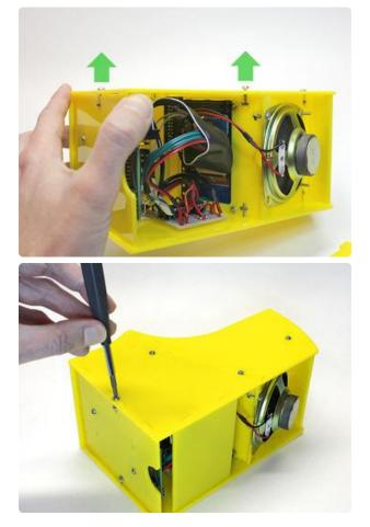
To install the back piece, you'll need to loosen two screws: the bottom and rearmost positions.
