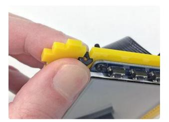
Feed a nut into the cross part of the "T," holding it in place between thumb and forefinger.
