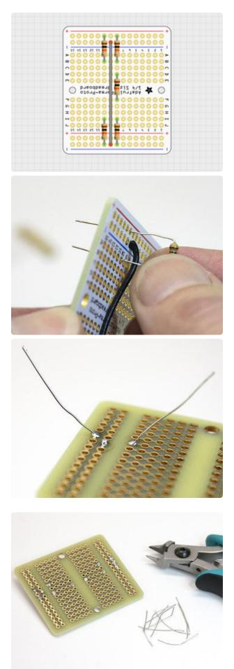
Install five 10K resistors (brown-blackorange) in the positions shown, immediately to the left and right of the ground wire. Two go on the left (audio) side, three on the right (joystick) side.
