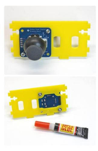
Install the joystick on its support piece, whichever one you selected (centered or off-center). Two screws at opposite corners are sufficient.
