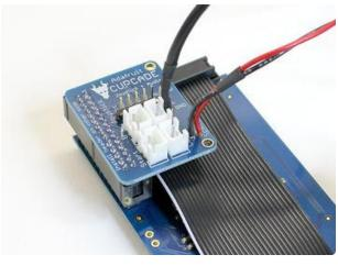
The board should be oriented to sit behind the PiTFT and ribbon cable, not hanging out over the side.
