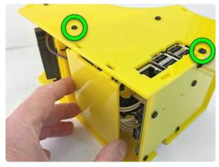
Get all the wires stuffed inside the case. Check the joystick jumper wires, which may have pulled free.
