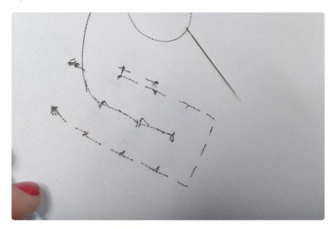
Keep power and ground lines far apart from each other. A short between power and ground will prevent your project from working and may even cause your battery to heat up.
