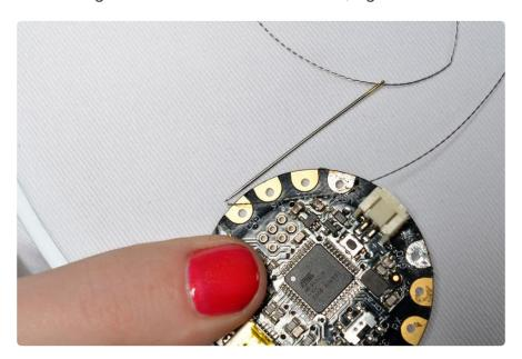
Pull the needle all the way through and continue pulling the thread tail until only 6 inches remains at the back of the fabric.
