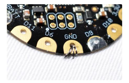
Repeat with a few more stitches to make a secure mechanical and electrical connection.
