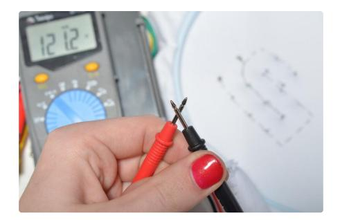
Use a multimeter's continuity tester to check your circuit for shorts. The meter will beep any time the two probes are electrically connected.
