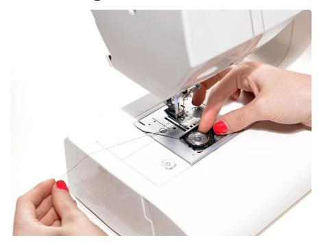
You can use our 2 ply conductive thread in the bobbin of a sewing machine. Thread the machine's needle with plain thread.
