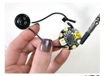
Bend the speaker's other wire to the Vout pin on GEMMA and solder in place.
