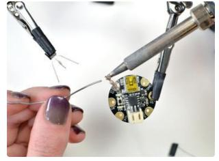
Next it's time to connect up the center leg of the transistor.
