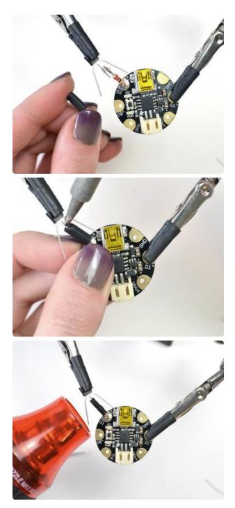
Don't forget heat shrink tubing! Cut a small piece of the medium size and place it over the resistor.
