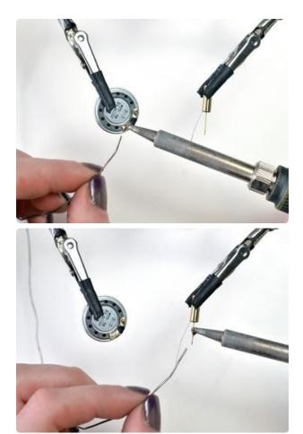
Place the small speaker and tilt ball switch in the jaws of a helping hand tool.
