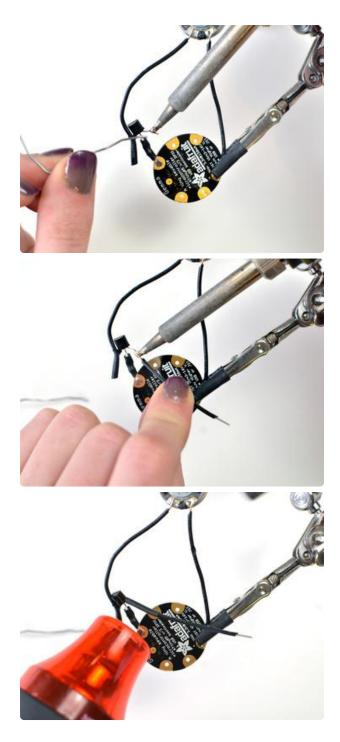
Tin the last remaining lead of the transistor and solder to a piece of wire. Slide on some heat shrink and use a heat gun to shrink it.
