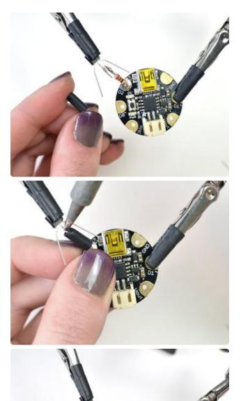
Don't forget heat shrink tubing! Cut a small piece of the medium size and place it over the resistor.
