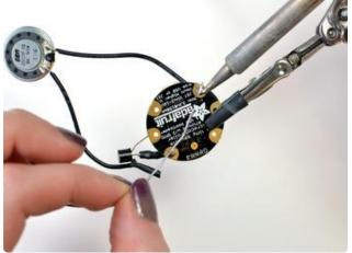
Bend the speaker's other wire to the Vout pin on GEMMA and solder in place.
