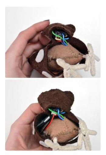
Because the GEMMA sits inside the tail of the owl, we needed to cut an additional tail piece from the brown felt included in the owl kit, then sewed it to the original tail piece to make a pocket.
