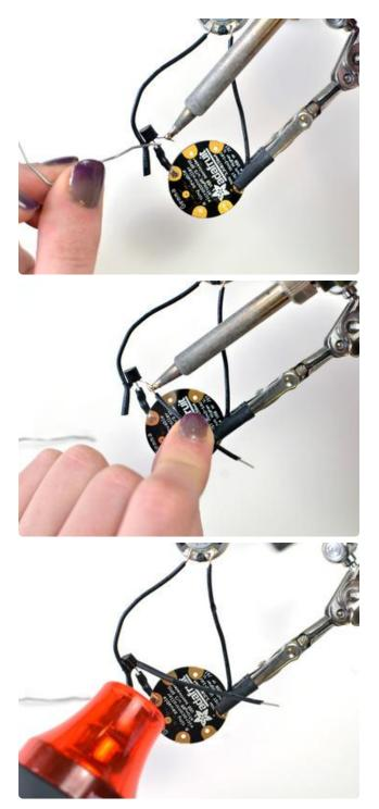
Tin the last remaining lead of the transistor and solder to a piece of wire. Slide on some heat shrink and use a heat gun to shrink it.
