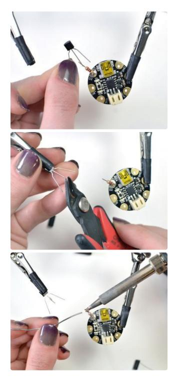
Next it's time to connect up the center leg of the transistor.
