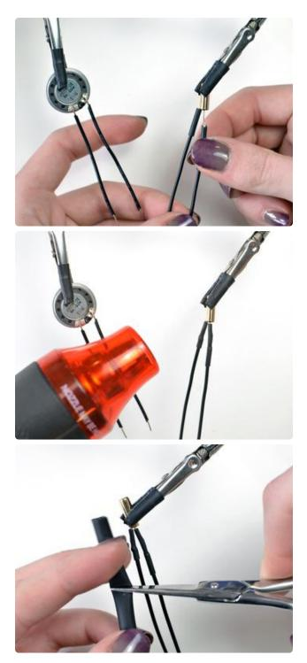
Slide a piece of the smallest diameter heat shrink tubing over each leg of the tilt ball switch to insulate the wires and solder connections.
