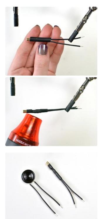
Your speaker and tilt ball switch are now ready for attaching to the rest of your circuit!
