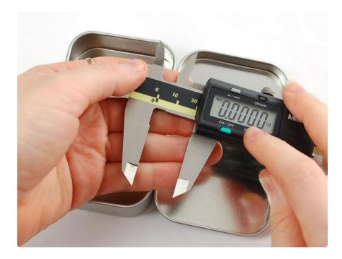
And measure the overall thickness. The difference is the thickness of the bottom metal.
