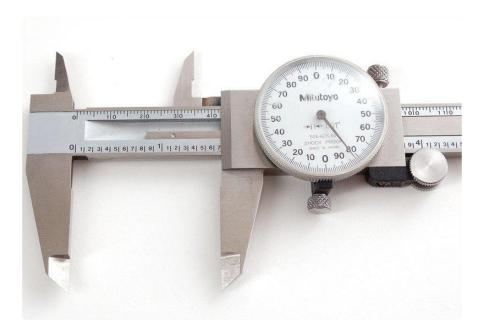
Dial calipers use a mechanical system consisting of a rack and pinion, there's a gearset inside as well that moves the dial in increments of one thousandth of an inch (or hundredth of a mm). To read, the 'most significant' value is read from the rule and the fractional value from the dial. The nice thing about dial calipers is that they don't use batteries and although are not waterproof, work well even if damp.
