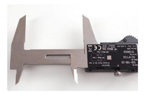
Digital calipers don't have any rack/pinion/gear system. This makes them more shock-proof which we like (since we're a little clumsy and have dropped the calipers a few times).
