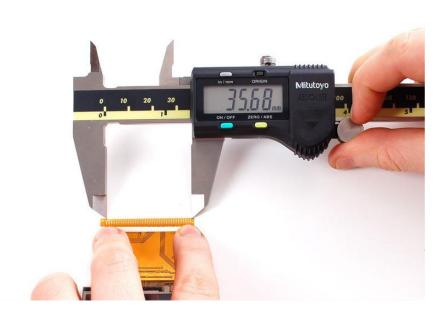
Remember that for a N pin connector, there are N-1 'gaps' (a common-enough confusion that it has its own name, the <u>fencepost-error</u> (https://adafru.it/aJ9) ) so divide 35.68mm by 36 = 0.99mm. Since we're eyeballing the center points of the connector, this should be rounded up to a 1mm pitch. Sometimes the number should be rounded up/down in imperial so if it seems off, check other units.
