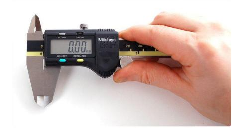
Before using your calipers, check that the origin is correct, clean the blades with a cloth to make sure there's no dust or dirt that would give the wrong measurement and close the jaws. You should read 0.0mm, if not, check that they're clean and if so, press the origin button. We've never had to do this since they are pre-origin'd at the factory but hey, you never know.
