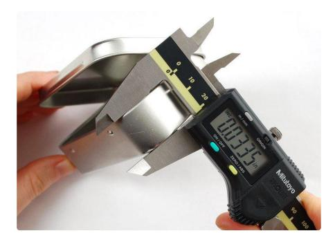
This measurement came out to 33.5 mils. The closest standard sheet gauge (https://adafru.it/aJ8) to 0.0335 is 20 gauge. Variations in the metal thickness may be due to additional thickness from the plating process or the rounded edges interfering with the depth measurement. Taking multiple measurements is always a good idea!
