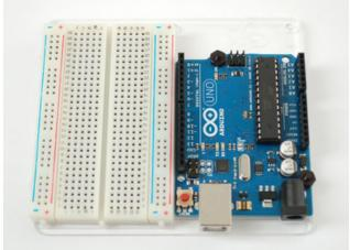
Remove the paper backing from the half size breadboard and stick it on next to the Arduino.
