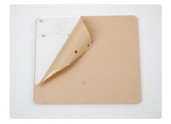
Start by peeling the paper backing off of the plastic plate. Begin at a corner, it should come off easily.
