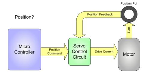
The Feedback Servos allow you to close this outer loop by providing the feedback signal to the microcontroller too!
