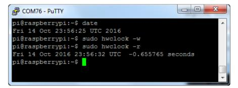
Once the time is set, make sure the coin cell battery is inserted so that the time is saved. You only have to set the time once
