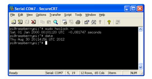
First you'll need to get the right time set on the Pi, the easiest way is to connect it up to Ethernet or Wifi - it will automatically set the time from the network. Once the time is correct (check with the date command), run sudo hwclock -w to write the system time to the RTC
