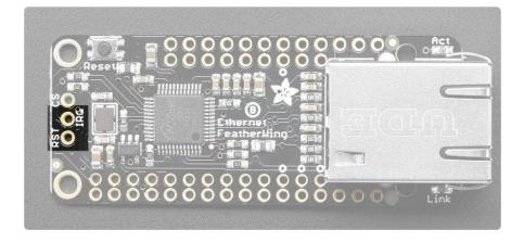
You can also connect to and use the IRQ and WIZ ReSeT pins. These are not used in the library and are there for advanced usage. They are 3.3V logic, 5V tolerant.
