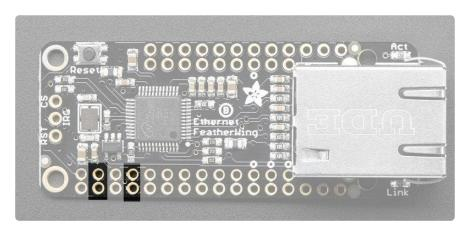
The WIZ5500 Ethernet chip (and really any ethernet chip) are fairly high current devices, requring about 150mA whether or not actively transmitting. The chip is powered from the 3.3V and GND pins indicated and does not have an internal regulator.
