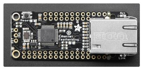
The Ethernet FeatherWing plugs into any Feather and adds hard-wired networking. To make it as cross-platform compatible as possible, we use only SPI plus one extra, configurable pin. It's not going to be gigabit (or even multi-megabit) speeds but it will work!
