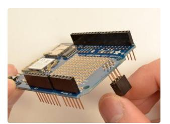
Insert the 2x3 stacking header as shown.
