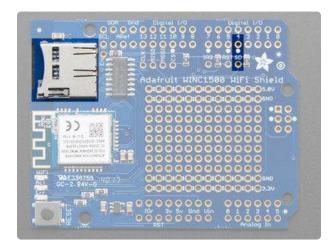
There's a lot of space available on this shield so we also stuck on a micro SD card holder, great for datalogging or storing data to transmit over WiFi.
