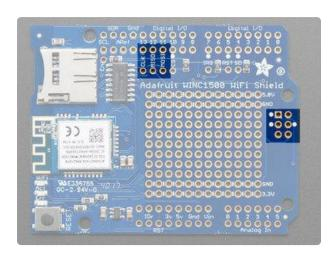
Both WiFi and SD card use SPI to send and receive data. These pins are labeled CLK MISO MOSI and have level shifting so you can use this shield with 3.3V or 5V microcontroller boards.
