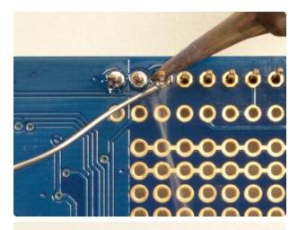
Once you've tacked and straightened all the headers, go back and solder the remaining pins for each header.
