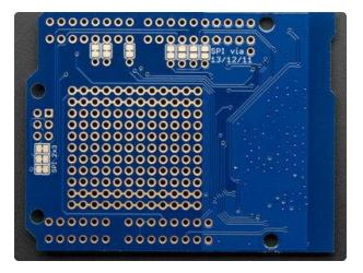
If you happen to want to use 11/12/13 rather than the SPI header, turn the board over, you can cut the 3 jumpers next to the 2-3 ISP header and solder the open jumpers between the SPI pins and D11/12/13
