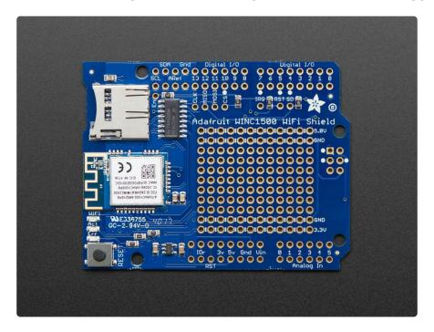
The Adafruit ATWINC1500 WiFi Shield uses SPI to communicate plus some GPIO for control, so with about 6 wires, you can get your wired up and ready to go. Right now
