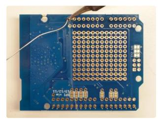
Tack one pin of each header, to get them set in place before more soldering. If the headers go crooked you can re-heat the one pin while re-positioning to straighten them up
