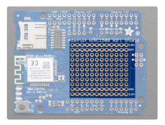
We have a big grid of prototyping holes and power rails if you want to make some custom circuitry!
