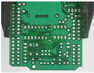
Use your diagonal cutters to clip the leads off just above the solder joint.
