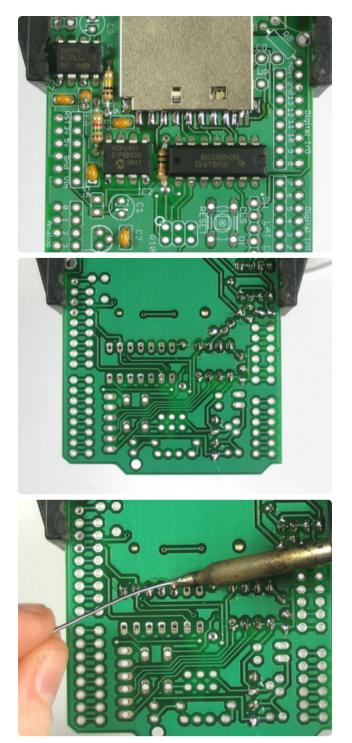
Next is **IC4**, the buffer to talk to the SD card. Match up the notch just like you did with the smaller chips.
