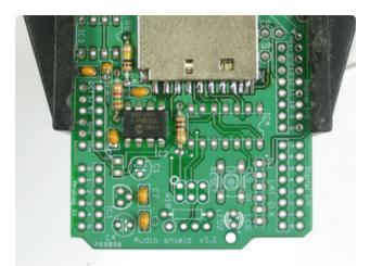
Next is the DAC (digital-analog converter) IC2. This is what turns the data into music. Make sure you pick the DAC to solder in here, it says MCP4921 on it and has a stylized M.
