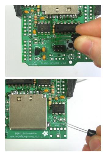
Next are the three electrolytic capacitors **C1 C4** and **C9**.
