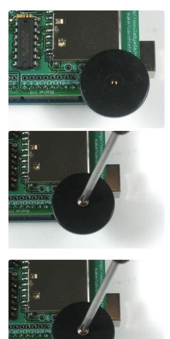
Next you can install the thumbwheel. Use a #0 screwdriver. Align the thumbwheel so it 'grabs' the potentiometer, then gently screw it in place.
