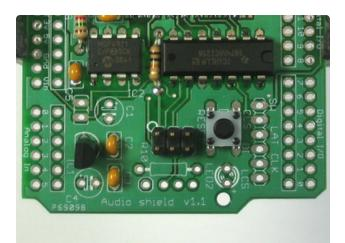
Next is the reset button and the ICSP header. These let you reset the Arduino manually, and reprogram it directly with a AVR programmer.
