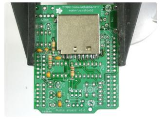
Once you're sure you have **C8** correct, you can place the remaining 0.1uF ceramic capacitors **C2**, **C3**, **C5**, **C6** and **C7**.
