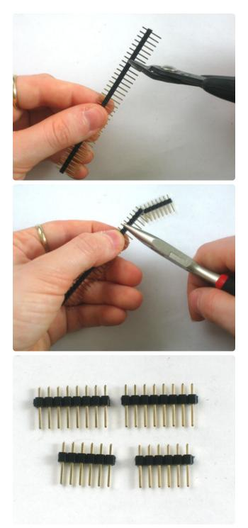
Next, break the 36-pin header strip into smaller sections so that the shield can be placed on the Arduino. You can use pliers or diagonal cutters. Clip off 2-6pin and 2-8pin pieces.
