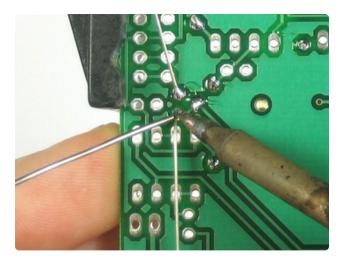
Solder and clip the small capacitor leads.
