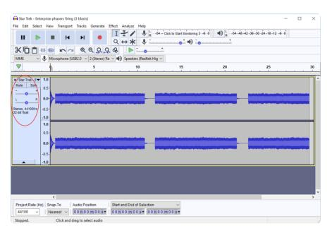
See the red circled text. That shows that the WAV file I chose is a 44.1 KHz, 32 bit stereo file which is above our microcontroller specifications noted (22 KHz, 16 bit, mono). We'll need to tell Audacity what parameters we want to convert the file.
