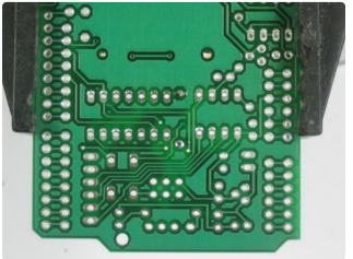
Use your diagonal cutters to clip the leads off just above the solder joint.
