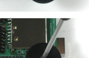
Next you can install the thumbwheel. Use a #0 screwdriver. Align the thumbwheel so it 'grabs' the potentiometer, then gently screw it in place.
