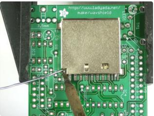
We'll start with the four side tabs that are used to mechanically secure the card holder in place.
