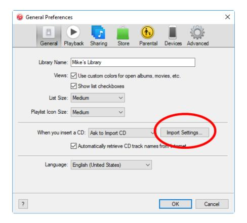
Then click Import Using: WAV Encoder, Setting Custom. In the new popup window, select Sample Rate: 22,050 kHz, Sample Size: 16-bit, Channels: Mono.
