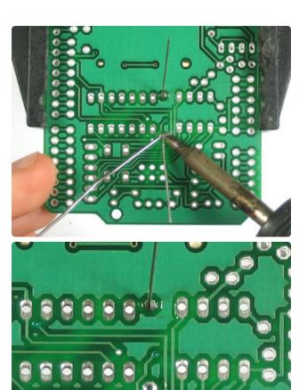
Solder the leads to the pads (metal ring) by heating both with the side-tip of the iron for 3 seconds and then poking in a bit of solder.
