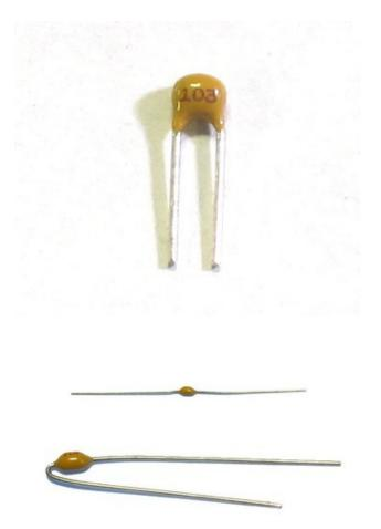
Next is the 0.01uF ceramic capacitor **C8**. The tricky part here is that in older kits there are many 0.1uF ceramic capacitors in the kit that look identical to the 0.01uF!
