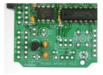
Next is the 3.3V regulator **IC1** that provides a nice powersupply to run the SD card. The regulator comes in a semi-circular package, so make sure it matches up with the silkscreened image.
