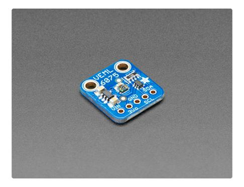
This little sensor is a great way to add UVA and UVB light sensing to any microcontroller project. The VEML6070 from Vishay has both true UVA and UVB band light sensors and an I2C-controlled ADC that will take readings and integrate them. The sensor also comes with calibration registers so you can easily convert the UVA/UVB readings into the UV Index.
