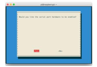
Keep the Serial Port Hardware enabled
