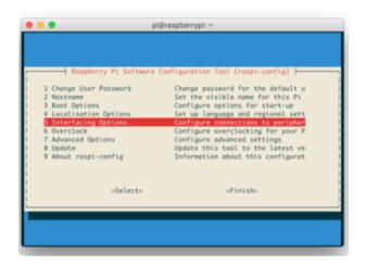
Run sudo raspi-config to open up the configuration page and select Interfacing Options or Advanced Options (it may be one or the other)
