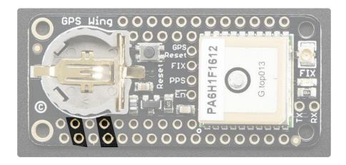
The GPS module runs from +3.3V power and uses 3V logic. the GPS is powered directly from the 3V and GND pins on the bottom left of the Feather. Each Feather has a regulator to provide clean 3V power from USB or battery power.
