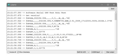
You can configure the GPS output you see by commenting/uncommenting lines in the setup() procedure. For example, we can ask the GPS to send different sentences, and change how often it sends data. 10 Hz (10 times a second) is the max speed, and is a lot of data. You may not be able to output "all data" at that speed because the 9600 baud rate is not fast enough.
