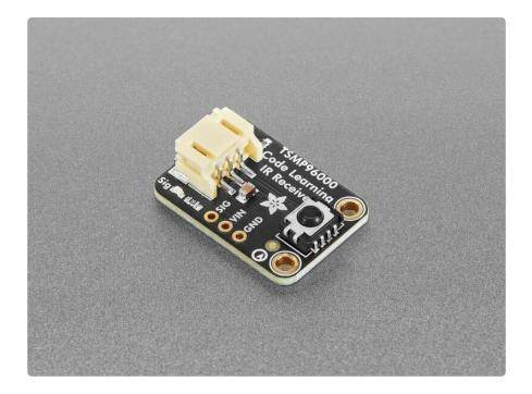
Each STEMMA board is a fully assembled and tested PCB, but no cable. No soldering is required to use it, but you will need to pick up <u>a 2mm pitch, 3-pin STEMMA JST PH</u> <u>cable (https://adafru.it/18cS)</u>. Alternatively, if you do want to solder, there's a 0.1" spaced header for power/ground/signal.
