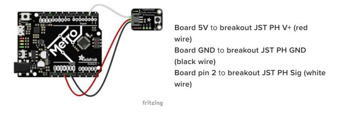
Here is an Adafruit Metro wired up using a solderless breadboard:
