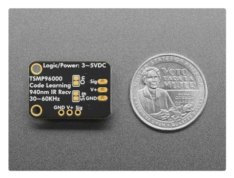
This board will work nicely for advanced IR remote receiving projects, because you don't get the demodulated output it's not good for most IR decoding firmware - make sure you've got code specifically designed for "code learning"! With mounting holes and a cable, it's easy to mount in enclosures and on devices. Using a 2mm pitch STEMMA JST PH cable with headers or alligator clips on the end, you can easily wire this board without any soldering.
