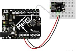
Board 5V to breakout VIN (red wire) Board GND to breakout GND (black wire) Board pin 2 to breakout SIG (white wire)
