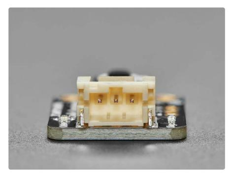
Usage is simple: Power the board by connecting V+ and ground to 3~5VDC, point a 20~60KHz IR remote control at the sensors, and press some buttons. The modulated IR signal, with the carrier signal intact, is piped out the Signal pin into your microcontroller which will then need to decode it. To make usage really easy, we have a green 'power good' LED and a red 'signal' LED. When IR remote signals are read by the onboard sensors, the red LED will blink to let you know.
