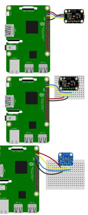
Pi 3V3 to sensor VIN (red wire on STEMMA QT version) Pi GND to sensor GND (black wire on STEMMA QT version) Pi SCL to sensor SCK (yellow wire on STEMMA QT version) Pi SDA to sensor SDA (blue wire on STEMMA QT version)
