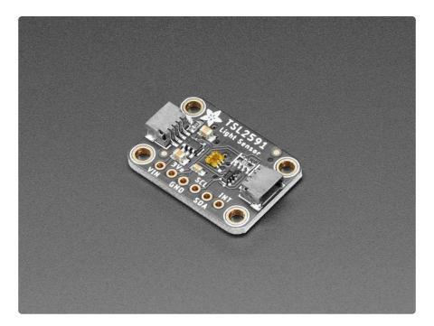
When the future is dazzlingly-bright, this ultra-high-range luminosity sensor will help you measure it. The TSL2591 luminosity sensor is an advanced digital light sensor, ideal for use in a wide range of light situations. Compared to low cost CdS cells, this sensor is more precise, allowing for exact lux calculations and can be configured for different gain/timing ranges to detect light ranges from up to 188uLux up to 88,000 Lux on the fly.
