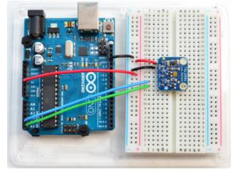
Connect Vin to the power supply, 3-5V is fine. (red wire on STEMMA QT version)
