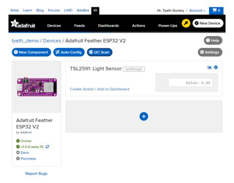
To view the data that has been logged from the sensor, click on the graph next to the sensor name.
