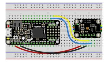
Board 3V to sensor VIN (red wire on STEMMA QT version) Board GND to sensor GND (black wire on STEMMA QT version) Board SCL to sensor SCL (yellow wire on STEMMA QT version) Board SDA to sensor SDA (blue wire on STEMMA QT version)
