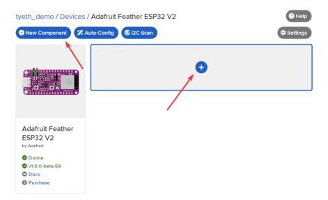
Adafruit IO supports a large amount of components. To quickly find your sensor, type TSL2591 into the search bar, then select the TSL2591 component.
