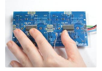
For a more robust connection, use a small bare wire across the pads instead of just solder. The legs trimmed off the LEDs are perfect for this!
