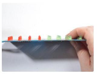
Check that the panels are aligned by looking from the side, gently bend/reheat until they are nice and straight
