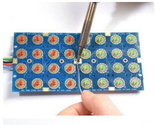
You can add a little more mechanical stability by soldering the large front tabs as well
