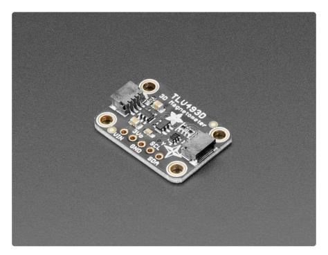
We've also outfitted the breakout with <u>SparkFun Qwiic</u> (https://adafru.it/Fpw) compatible <u>STEMMA QT</u> (https://adafru.it/Ft4) connectors to allow you to use it with other similarly equipped boards without needing to solder. Because the TLV394D "speaks" I2C, you only need two wires (in addition to power) to interface with your
