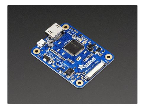
You can even power the display and decoder from a USB port. For example, with a 5" 800x480 display and 50mA backlight current, the current draw is 500mA total. You can reduce that down 370mA by running the backlight at half-brightness (25mA). With the backlight off, the decoder and display itself draws 250mA. If you want more backlight control, there's a PWM input, connect that to your microcontroller or other PWM output and you can continuously dim the backlight as desired
