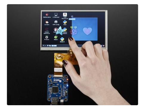
If you purchased the version of the decoder with touch support, you will receive a decoder board with extra circuitry for a resistive touch screen decoder. The circuit is an AR1100 USB resistive touch driver, so it basically just uses the same USB port you use to power, but for the data
