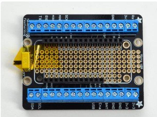
If you'd like to install the slide on/off switch, snap it into place at the end of the PCB and tape it down so it doesn't fall out when soldering
