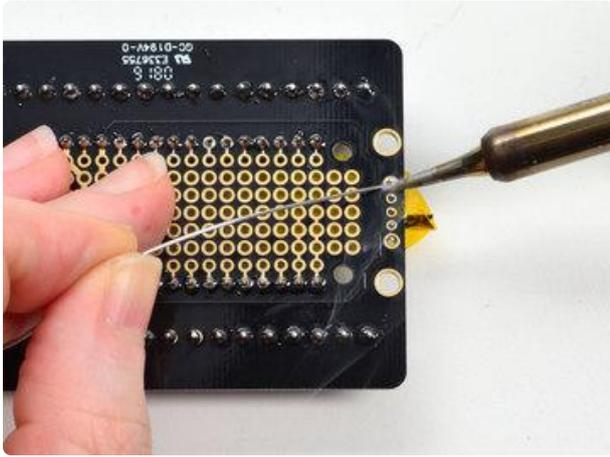
Solder in the two large mechanical points and the three signal pins in the center
