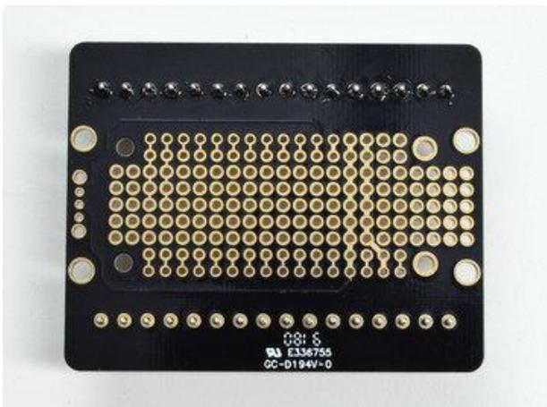
Check the first row once its done, to make sure each pin is shiny and completely soldered
