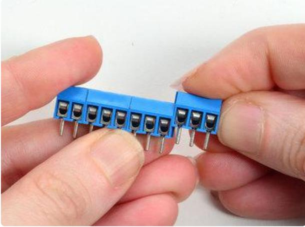
Keep sliding more 3-pin blocks on until you get a 2-pin block with four 3-pin blocks in the middle and then another 2-pin block at the end
