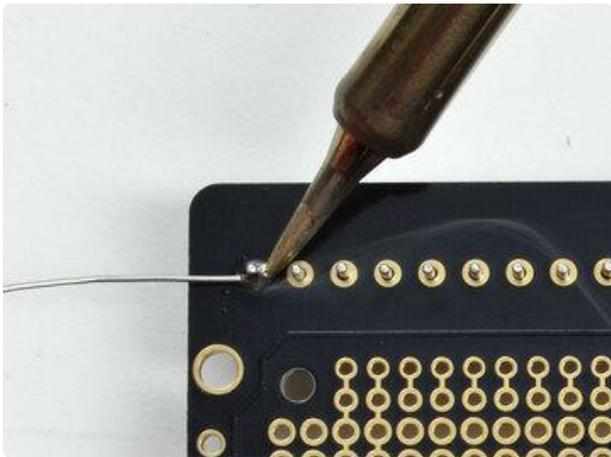
Flip over the board and solder in all of the terminal block pins with plenty of solder
