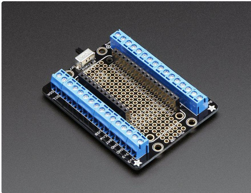
The Terminal Block Breakout FeatherWing kit is like the Golden Eagle of prototyping FeatherWings (eg. majestic, powerful, good-looking). To start, you get a nice prototyping area underneath your Feather, with extra pads for ground, 3.3V and SDA/SCL. Not one to stop there, we expanded the PCB out to 2" x 2.5" with 3.5mm pitch terminal blocks down each side. There's also four mounting holes so you can attach the breakout to your enclosure or project.
