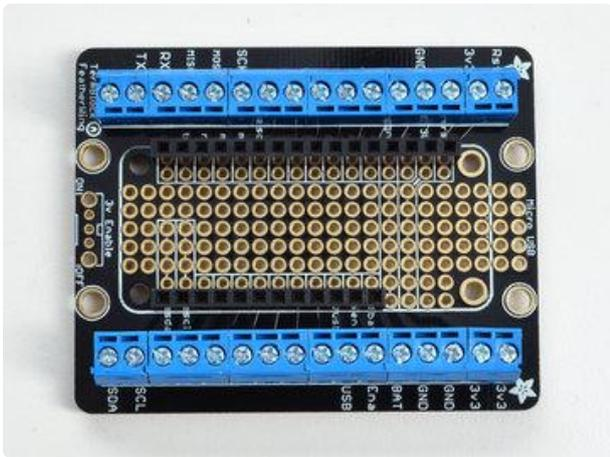
Next up place the 12-pin and 16-pin headers in the center part of the breakout in the outer-most set of holes
