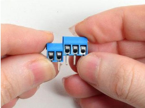
Start by grabbing the blue terminal blocks. Terminal blocks only come in 2 and 3 pin sizes, but can be slid together to form longer strips. Start by connecting a 2 and 3 pin piece together. There's nubs on either side so line those up and you'll be able to slide them together
