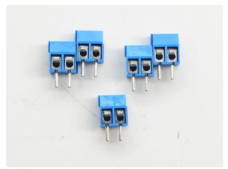
Next we will solder in the five 3.5mm terminal blocks used to connect power & the motors to the FeatherWing board.
