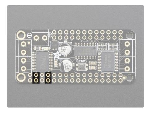
The logic power to the I2C expander and motor pins comes from the Feather's 3.3V regulator, 3.3V and ground are both required.
