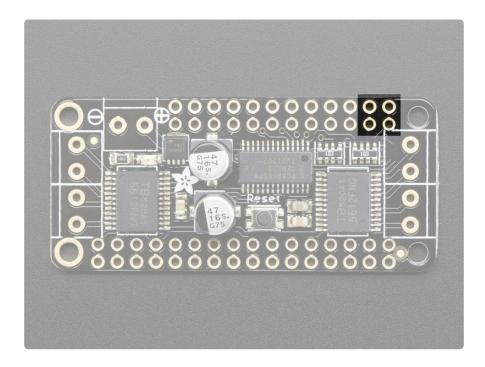
All data and control is done over I2C so it works with any and all Feathers! No need to set any PWMs. SDA and SCL are highlighted above. There are 10K pullups to 3.3V on each.
