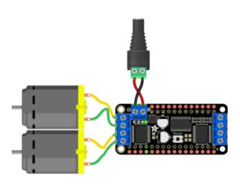
Connect the two motor wires from the first motor to the M1 terminal on the FeatherWing.
