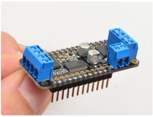
The terminal blocks have interlocking dovetailed grooves on the sides. Line two of them up as shown, and press down to lock them together as a 4-position terminal block. It is a snug fit, so you may have to press hard.
