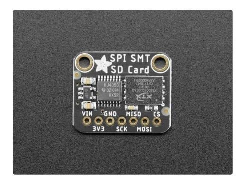
We made this breakout to be a quickstart for this chip. We wired the chip in "SPI" mode, with a level shifters so you can use it with 3V or 5V logic easily. You also get a 3.3V regulator and a pullup on CS. Wire up the SPI pins to your microcontroller, use your favorite SD library and you'll be ready to rock in minutes!
