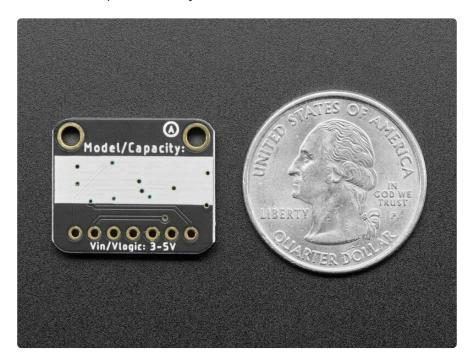
Compared to plain SPI flash, this NAND memory chip handles all the wear leveling and ECC calculation. You don't have to manually erase blocks, you just write and read them like you would with any SD card. You can clock it up 50 MHz and the 'write speed class' is 8 (although you may not be able to get that fast with plain 1-bit SPI compared to SDIO).
