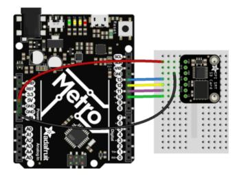
Arduino 5V to breakout VIN
