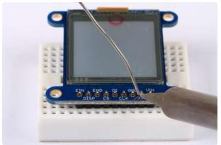
Solder! Solder each pin to assure good electrical conductivity.
