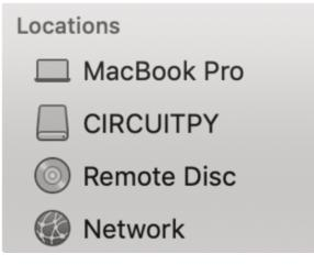
After it finished uploading, and with the Circuit Playground board connected over USB, it should appear on your computer as a flash drive called CIRCUITPY.
