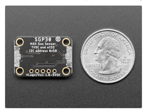
This part will measure eCO2 (equivalent calculated carbon-dioxide) concentration within a range of 400 to 60,000 parts per million (ppm), and TVOC (Total Volatile Organic Compound) concentration within a range of 0 to 60,000 parts per billion (ppb).
