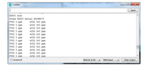
The first 10-20 readings will always be TV0C 0 ppb eC02 400 ppm. That's because the sensor is warming up, so it will have 'null' readings.
