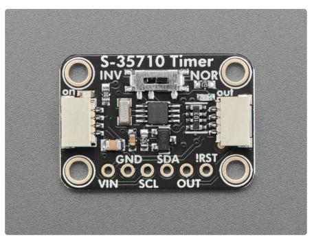
The Adafruit S-35710 Wake Up Timer is a low power 'watchdog timer' chip that can be programmed to alert with a digitally-configurable alarm from 1 second up to 194 days, thanks to a 24-bit seconds counter.
