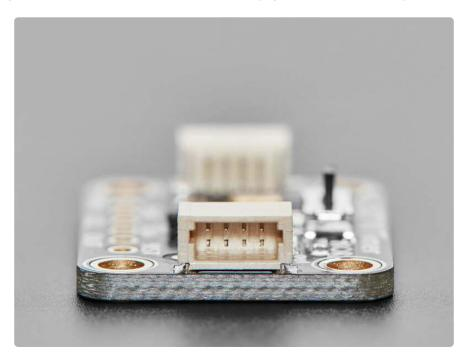
One thing to note is that on power-up the OUT line is default low, which means its not good for a low-power sleep manager, only for watch-dog-like timings. That is to say, you cannot connect this to your microcontroller's reset or enable line to self-depower because it will be disabled/reset when powered up.
