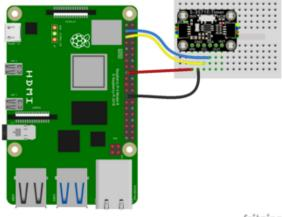
Pi 3V to breakout VIN (red wire) Pi GND to breakout GND (black wire) Pi SCL to breakout SCL (yellow wire) Pi SDA to breakout SDA (blue wire)
