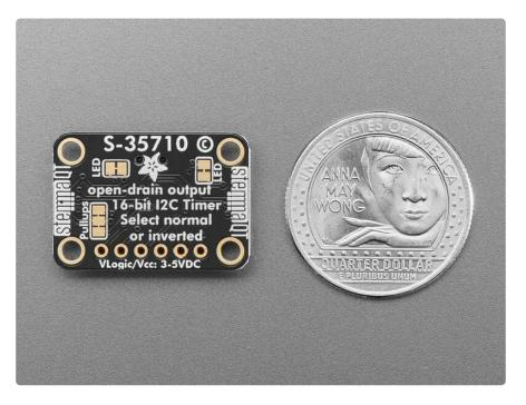
Usage is pretty simple: on I2C write of the timer register, the chip starts counting from 0 seconds up and the OUT pin goes high. When the count matches the timer register, the OUT pin goes low.
