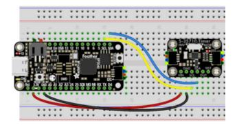
Board 3V to breakout VIN (red wire) Board GND to breakout GND (black wire) Board SCL to breakout SCL (yellow wire) Board SDA to breakout SDA (blue wire)
