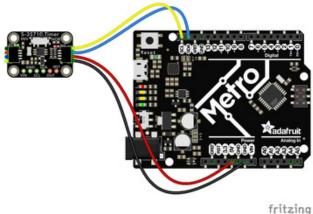
Board 5V to breakout VIN (red wire) Board GND to breakout GND (black wire) Board SCL to breakout SCL (yellow wire) Board SDA to breakout SDA (blue wire)
