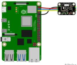
Pi 3V to breakout VIN (red wire) Pi GND to breakout GND (black wire) Pi SCL to breakout SCL (yellow wire) Pi SDA to breakout SDA (blue wire)
