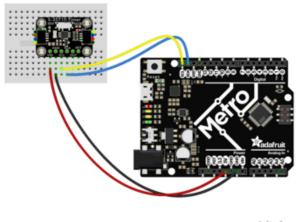
Board 5V to breakout VIN (red wire) Board GND to breakout GND (black wire) Board SCL to breakout SCL (yellow wire) Board SDA to breakout SDA (blue wire)
