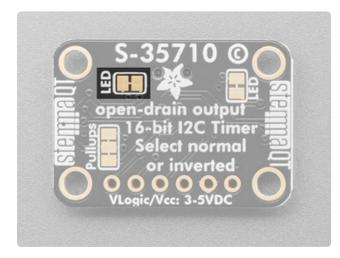
Output LED - In the upper right corner, behind the STEMMA connector, on the front of the board, is the output LED, labeled out. It is a red LED. This LED will be on when the OUT pin is low and off when the OUT pin is high. LED jumper - This jumper is located on the back of the board, to the left of the Adafruit logo on the board silk. Cut the trace on this jumper to cut power to the "out" LED.
