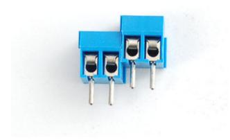
Find the terminal blocks, they're blue and come in 3-pin and 2-pin shapes. We'll need to slide the blocks together for the next step where we put the blocks into the proto plate. Slide them together to make 1x8 pin, 1x5 pin, and 3x4pin terminal blocks
