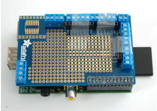
This part is optional, but if you want to have sockets for the GPIO pins so you can plug wires in and out easily, you can solder in the two 8-pin and single 6-pin header.
