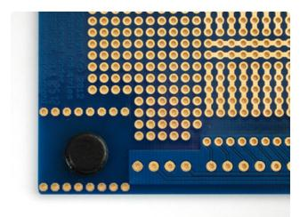
Place the single bumper underneath the SOIC breakout area. This will make the plate sit nicely on the Ethernet port
