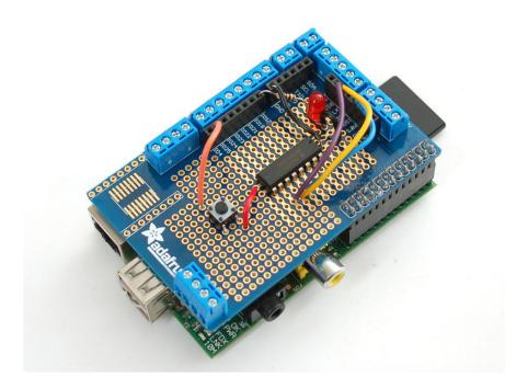
The terminal blocks make it easy to connect to wires for installations. Simply use a small Phiiips or flathead to open up the block, insert a stranded or solid core wire, then tighten it down.
