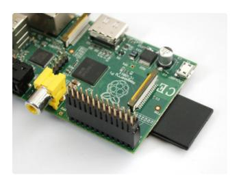
Place the big 2x13 pin header onto the Raspberry Pi GPIO breakouts so that it covers every pin. The connector is symmetric so it will fit on either way.
