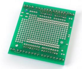
Solder all the pins of the header with plenty of solder.
