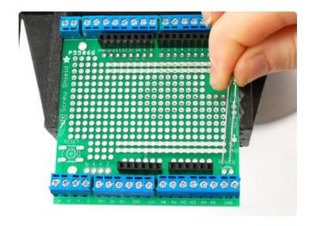
Next we'll place the two LEDs. The first LED is the green-colored one. This will tell us when the Arduino and shields are powered.
