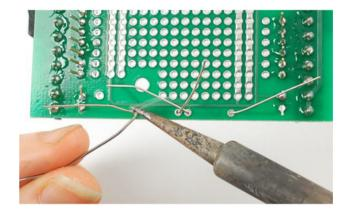
Solder and clip the two resistors.
