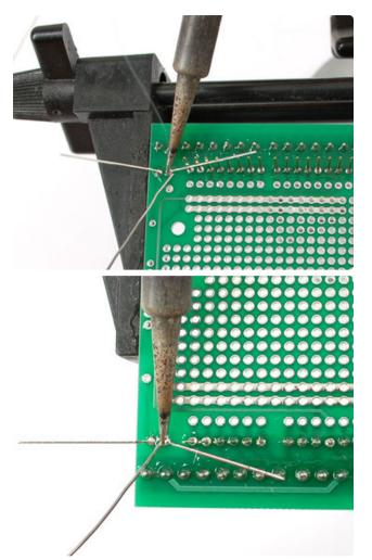
Solder both LEDs in place.
