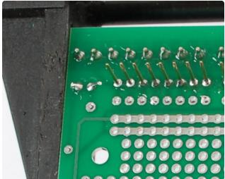
Use the diagonal cutters to clip the long LED legs. They should be cut just above the solder joint.
