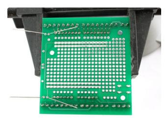
You can bent the LED leads out of the way to keep the LEDs flat against the PCB.
