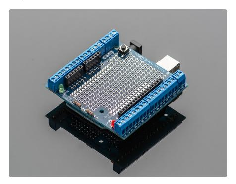
The shield even comes with <u>stacking headers</u>, (https://adafru.it/alH) which let you plug another shield on top! As shown here, a data logging shield is stacked onto the protoscrewshield.
