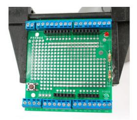
Last we will place the reset switch. This switch will let you easily reset the Arduino.
