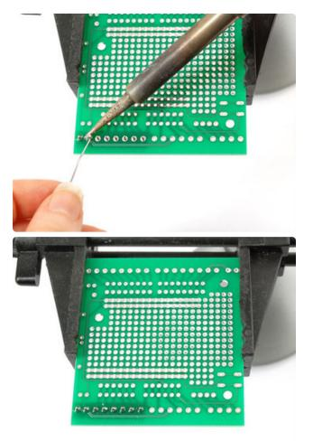
And solder the pins to the pads. Use plenty of solder so that you get the pads completely filled.
