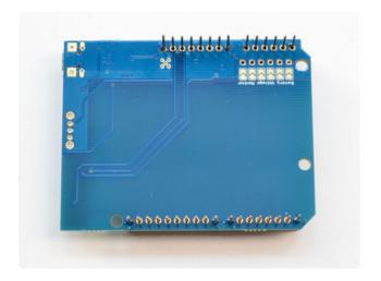
Carefully remove the shield from the Arduino and place flat on the table, long pins sticking up
