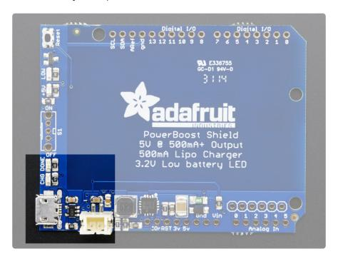
There's two LEDs next to the microUSB jack which will tell you how charging is going. If the CHG LED is on (yellow) that means its charging. the DONE LED (green) turns on when the battery is full.
