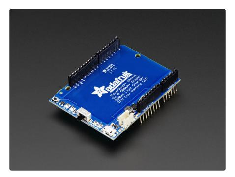
What's a project if it's trapped on your desk? Now you can take your Arduino anywhere you wish with the PowerBoost shield! This stackable shield goes onto your Arduino and provides a slim rechargeable power pack, with a built in battery charger as well as DC/DC booster.
