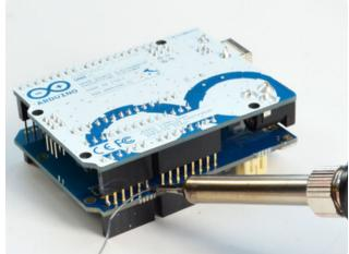
Tack the outer pins of each stacking header. This way they'll be aligned right.
