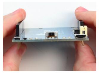
If you want to add the on/off switch, place the switch in the slot in the middle of the PCB
