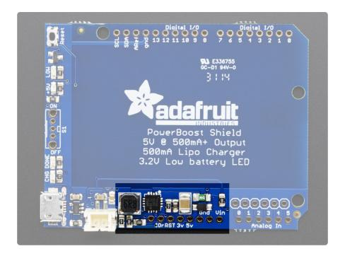
To protect the booster and battery, we put a 500mA fuse on the output of the boost section. The fuse will trip when a continuous current higher than 1A is detected.
