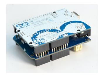
Check your work by looking to make sure the pins are soldered
