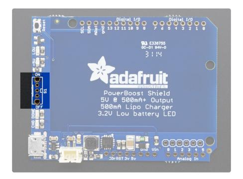
If you would like to custom attach your own switch, solder a switch to the middle pin and the pin right below the middle pin. Any voltage/current rating is fine as the switch is signal, not power, carrying
