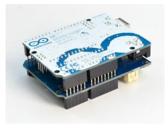
Pull on the shield a bit so that you get a few mm of gold pins showing, then flip it all over and place on a table as shown. It should sit nice and flat
