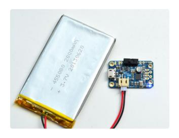
When the switch is to the left, the 5V power will be on, you can tell because the blue LED is lit
