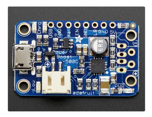
The PowerBoost 500C has at the heart a <u>TPS61090 boost converter from TI</u> (https://adafru.it/duQ). This boost converter chip has some really nice extras such as low battery detection, 2A internal switch, synchronous conversion, excellent efficiency, and 700KHz high-frequency operation. Check out these specs!
