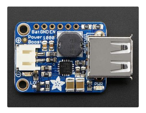
The PowerBoost 1000 has at the heart a <u>TPS61030 boost converter from TI</u> (https://adafru.it/dLY). This boost converter chip has some really nice extras such as low battery detection, 4A internal switch, synchronous conversion, excellent efficiency, and 700KHz high-frequency operation. Check out these specs!
