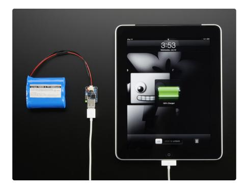
PowerBoost is the perfect power supply for your power-hungry portable project! This little DC/DC boost converter module can run from 1.8V batteries or higher, and convert that voltage to 5.2V DC for running your 5V projects. With a beefy 4A DC/DC converter, it can give you 1A+ from as low as 2V.
