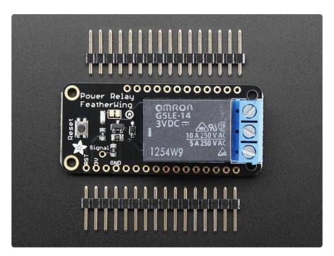
Each FeatherWing comes with a fully assembled and tested PCB, header you can use to attach to your Feather. By soldering closed the jumper on the underside of the Wing you can select which pin you want to use for the relay control. Some light soldering is required.
