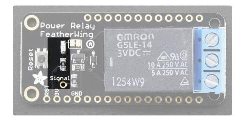
Controlling the relay is really simple. The relay uses a single pin for control. When floating or pulled low, the relay is 'open' or unset. When the pin is pulled high, the relay switches closed/set. A red LED next to the pin will let you know that the signal is high. You will need to solder closed a jumper on the bottom to match the pin you want to use for control.
