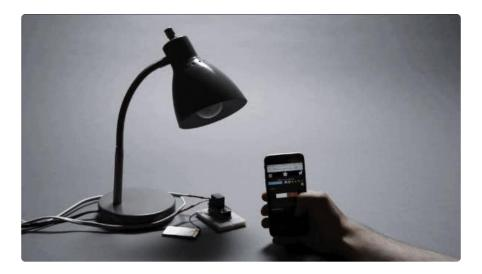
A Feather board without ambition is a Feather board without FeatherWings! This is the Power Relay FeatherWing. It gives you power to control, and control over power. Put simply, you can now turn on and off lamps, fans, solenoids, and other small appliances that run on up to 250VAC or DC power using any Feather board. Compared to our smaller mini Relay FeatherWings (https://adafru.it/xDL), this one can handle a beefy 1200 Watts!
