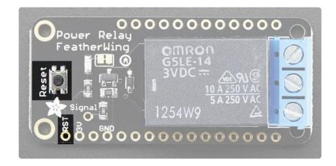
There is a Reset button on both Wings, this is connected to the RST pin and will short it to ground. It is not connected to the relay at all, its handy for restarting your Feather
