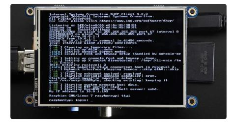
It's designed to fit nicely onto the Pi Model A or B but also works perfectly fine with the Model B+ as long as you don't mind the PCB overhangs the USB ports by 5mm.
