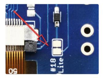
If you'd like to not have #18 control the backlight, simply cut the solder jumper, the tiny trace between the two large gold pads marked Lite #18
