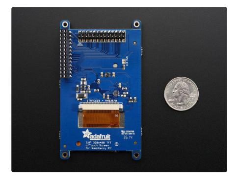
Best of all, it comes fully assembled and ready to plug into your Pi! You can use this as a display for running the X interface, or pygame. You can also have an HDMI display seperately connected.
