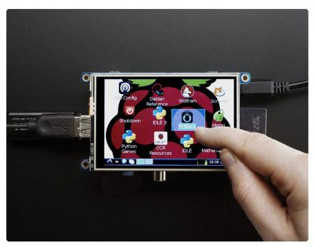
Is this not the cutest, little display for the Raspberry Pi? It features a 3.5" display with 480x320 16-bit color pixels and a resistive touch overlay, but is only slightly larger than <u>our popular original (https://adafru.it/dDE)</u>. The plate uses the high speed SPI interface on the Pi and can use the mini display as a console, X window port, displaying images or video etc. Best of all it plugs right in on top!
