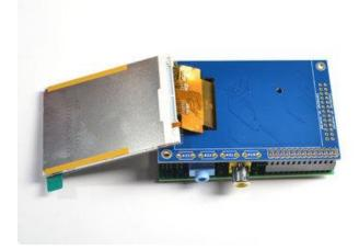
Place the PiTFT shield on top so all the pins stick through the connector on the side. Gently flip the TFT so its off to the side and wont be in your way while you solder
