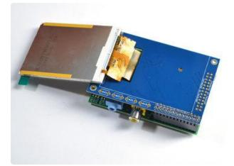
Before attaching the display, check that all the pins are soldered nicely and there's no bridging, cold solder, shorts, or unsoldered pins.
