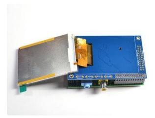
Place the PiTFT shield on top so all the pins stick through the connector on the side. Gently flip the TFT so its off to the side and wont be in your way while you solder
