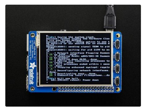
This design uses the hardware SPI pins (SCK, MOSI, MISO, CEO, CE1) as well as GPIO #25 and #24. All other GPIO are unused. Since we had a tiny bit of space, there's 4 spots for optional slim tactile switches wired to four GPIOs, that you can use if you want to make a basic user interface. For example, you can use one as a power on/off button.
