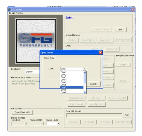
And press OK when done. You should see the following, with a blue success message and some device statistics in the bottom corner. You can change the baud rate in the bottom left hand corner, as well as the "security level" (how sensitive it is) but we suggest leaving those alone until you have everything running and you want to experiment. They should default to 57600 baud and security level 3 so set them if they're wrong
