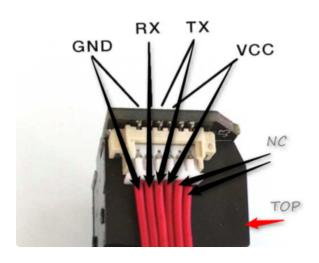
If your sensor is an older one and has all the same-color wires, The first wire from the left is ground, then the two data pins, then power. You'll have to cut, strip and solder the wires.
