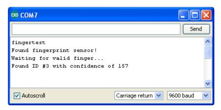
If you can't get 'connected' to the sensor the library says "Did not find fingerprint sensor :(" Try swapping the RX and TX wires and resetting
