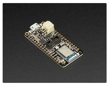
The Adafruit Feather nRF52 Pro is our latest Bluetooth Low Energy board for advanced projects and users who want to use a fully open source Bluetooth Low Energy 5.0 stack. It has a native-bluetooth chip, the nRF52832, as well as built in USB Serial and battery charging! We have other boards in the Feather family, check'em out here. (https://adafru.it/I7B)
