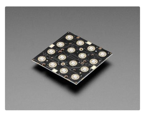
These 4x4 button pad boards are fully tile-able and communicate over I2C. With 5 address pins, you've got the ability to connect up to 32 together in any arrangement you like. With our trusty seesaw I2C-to-anything chip (https://adafru.it/Cmk), you don't
