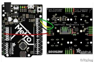
Wiring is easy, solder the four VIN GND SDA SCL pads to wires and then connect to your Arduino compatible:
