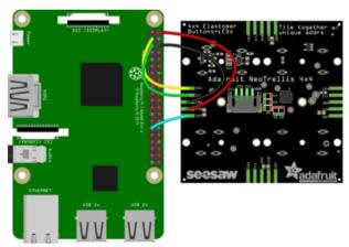
Wiring is easy, solder the four VIN GND SDA SCL pads to wires and then connect to your CircuitPython device
