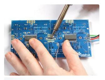
Use your soldering iron to drag solder from one pad to another, with a little effort they'll stick together and make a connection. You can add more solder to make the connection stronger. Its still not mechanically strong - so be careful not to bend or shake the arrangement
