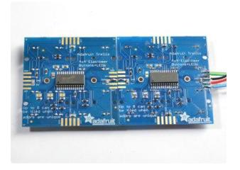
Solder two blobs of solder on two adjacent finger pads.
