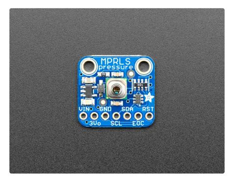
Unlike most ported pressure sensors, this one uses I2C, it's really easy to use with any microcontroller. Inside is a silicone-gel covered pressure sensing gauge with a pre-calibrated and compensated 24 bit ADC. We have example code and libraries for Arduino (https://adafru.it/CCe) or CircuitPython/Python (https://adafru.it/CCf). You can measure absolute pressure 0 to 25 PSI, which is a great range since ambient pressure here on Earth is about 14.5 PSI.
