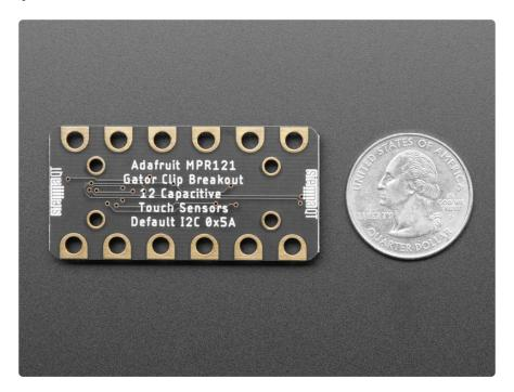
This sensor comes as a tiny hard-to-solder chip, so we put it onto a breakout board for you. Since it's a 3V-only chip, we added a 3V regulator and I2C level shifting so it's safe to use with any 3V or 5V microcontroller/processor like Arduino. We even added an LED onto the IRQ line so it will blink when touches are detected, making debugging by sight a bit easier on you.
