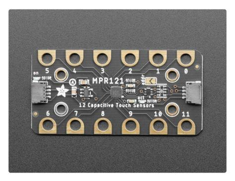
The MPR121 has support for reading data over I2C, which can be implemented with nearly any microcontroller. You can select one of 2 addresses with the ADDR pin
