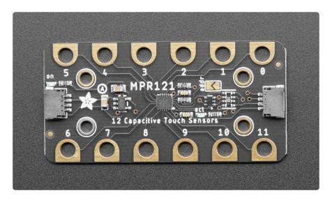
The little chip in the middle of the PCB is the actual MPR121 sensor that does all the capacitive sensing and filtering. We add all the extra components you need to get started, and you can connect to this board using STEMMA QT / QWIIC connectors. There are a series of 12 chonkpads for touch sensing with your finger or for easily connecting up alligator/croc clips.
