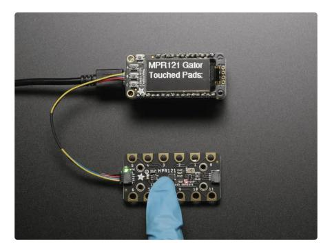
Add lots of touch sensors to your next microcontroller project with this easy-to-use 12-channel capacitive touch sensor breakout board, starring the MPR121. This chip can handle up to 12 individual touchpads with plug-and-play STEMMA QT connector and large alligator/croc-clip friendly pads, it's a no-solder solution to capacitive touch sensing.
