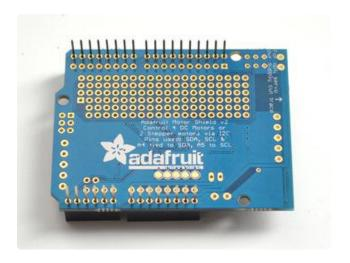
Start by sliding the 10 pin,  $2 \times 8$  pin and 6-pin stacking headers into the outer rows of the shield from the top. Then flip the board over so its resting on the four headers. Pull on the legs if necessary to straighten them out.
