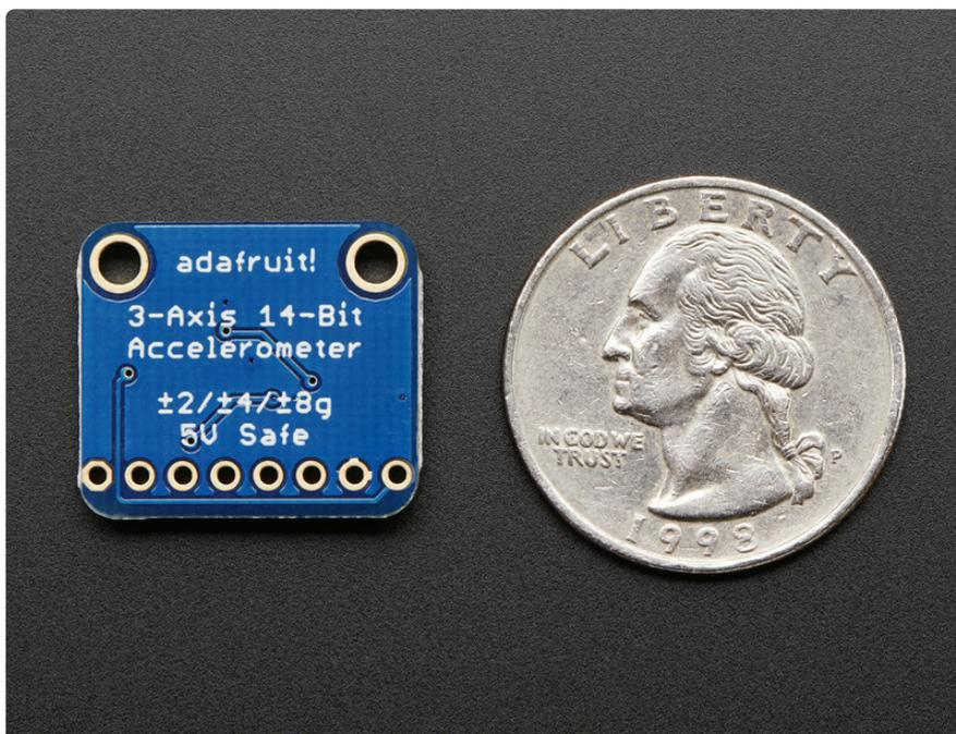
To get you going fast, we spun up a breakout board for this little guy. Since it's a 3V sensor, we add a low-dropout 3.3V regulator and level shifting circuitry on board. That means its perfectly safe for use with 3V or 5V power and logic.
