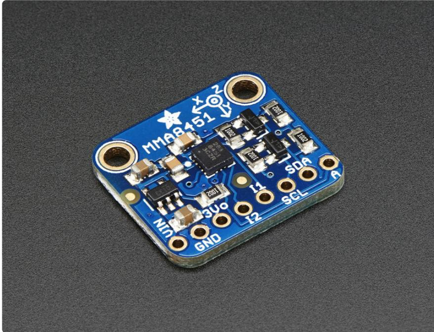
You can detect motion, tilt and basic orientation with a digital accelerometer - and the MMA8451 is a great accelerometer to start with. It's low cost, but high precision with 14-bit ADC. It has a wide usage range, from  $\pm 2g$  up to  $\pm 8g$  yet is easy to use with Arduino or another microcontroller
