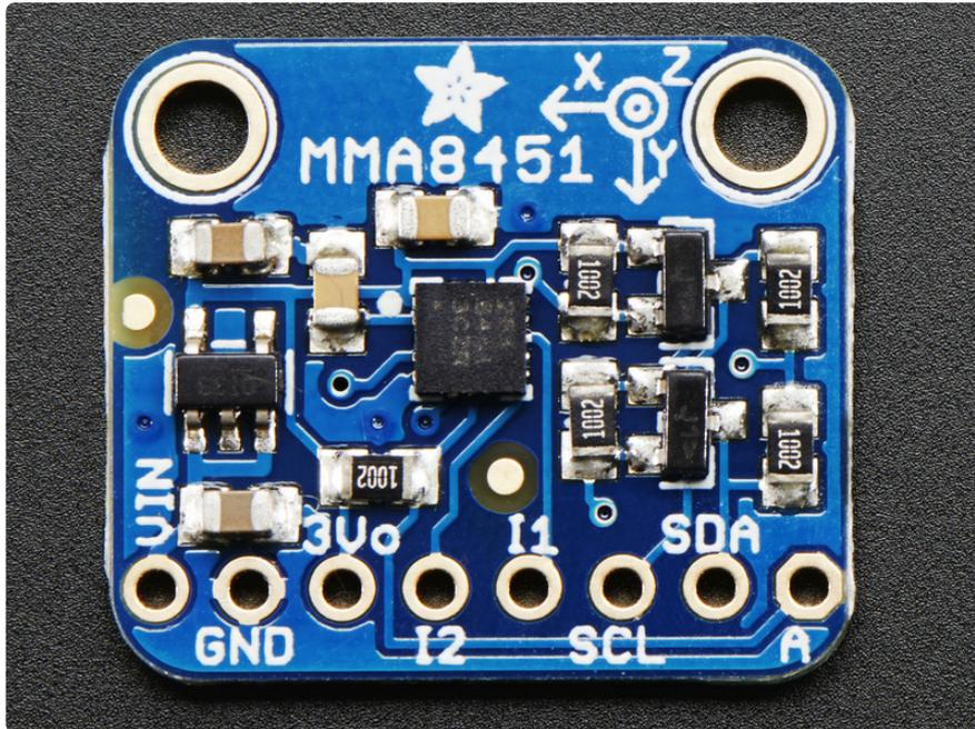
The little chip in the middle of the PCB is the actual MMA8451 sensor that does all the motion sensing. We add all the extra components you need to get started, and 'break out' all the other pins you may want to connect to onto the PCB. For more details you can check out the schematics in the Downloads page.
