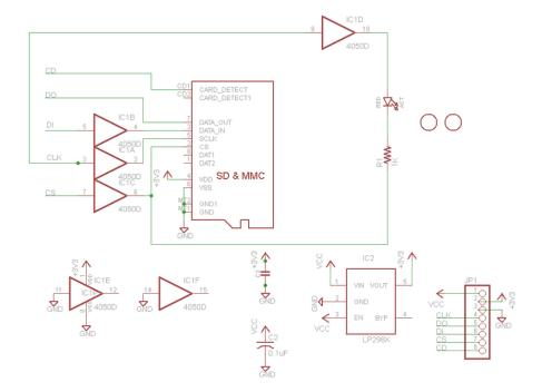
For the level shifter we use the  $\underline{\text{CD74HC4050}}$  (https://adafru.it/Boj) which has a typical propagation delay of ~10ns
