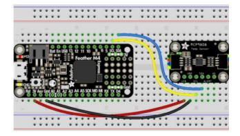
Board 3V to sensor VIN (Vdd) (red wire on STEMMA QT version) Board GND to sensor GND (black wire on STEMMA QT version) Board SCL to sensor SCL (yellow wire on STEMMA QT version) Board SDA to sensor SDA (blue wire on STEMMA QT version)
