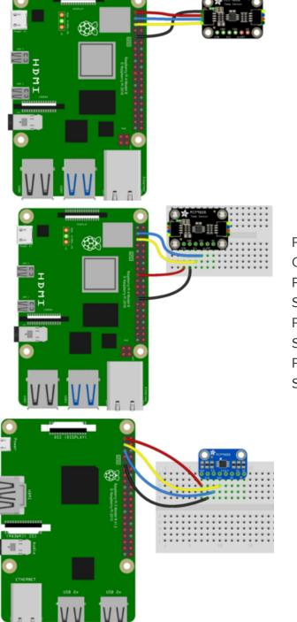
Pi 3V3 to sensor VIN (red wire on STEMMA QT version) Pi GND to sensor GND (black wire on STEMMA QT version) Pi SCL to sensor SCK (yellow wire on STEMMA QT version) Pi SDA to sensor SDA (blue wire on STEMMA QT version)
