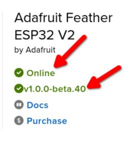
On the device page, quickly check that you're running the latest version of the WipperSnapper firmware.
