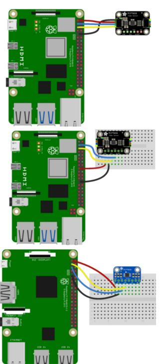
Pi 3V3 to sensor VIN (red wire on STEMMA QT version) Pi GND to sensor GND (black wire on STEMMA QT version) Pi SCL to sensor SCK (yellow wire on STEMMA QT version) Pi SDA to sensor SDA (blue wire on STEMMA QT version)
