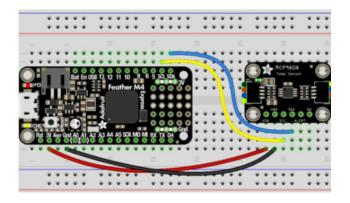
Board 3V to sensor VIN (Vdd) (red wire on STEMMA QT version)
