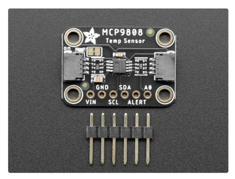
Unlike the DS18B20, this sensor does not come in through-hole package so we placed this small sensor on a breakout board PCB for easy use. The PCB includes
