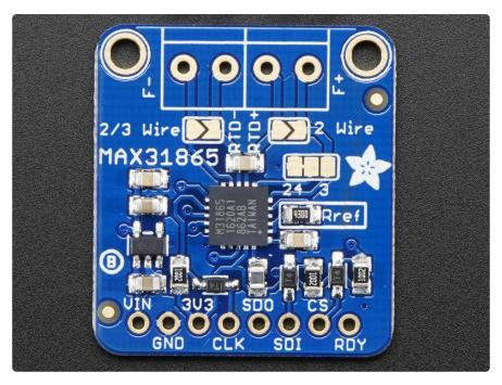
The MAX31865 is a tiny surface mount chip, and it needs a lot of other parts to make it work, so we've got it on a nice breakout board for you. You can control the chip and read data from it using the breakouts at the bottom. Let's go thru these!
