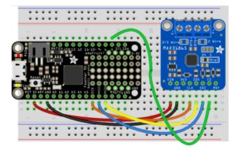
Board 3V to sensor VIN Board GND to sensor GND Board SCK to sensor CLK Board MOSI to sensor SDI Board MISO to sensor SDO Board D5 to sensor CS (or any other digital I/O pin)
