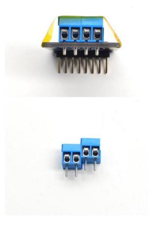
Make sure the open parts of the terminals face outwards so you can easily connect wires
