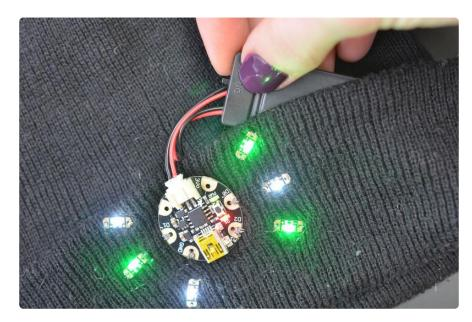
Once your program is doing what you like, unplug the USB cable and plug in a battery pack like our 2x2032 holder with on/off switch.
