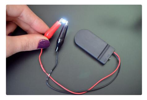
Simply connect 3 to 6VDC to the + pin and ground to the - pin, and the LED on the board will light up. In the photo above we've soldered alligator clips to a 2x2032 coincell battery holder (~6V). You could also use a single CR2032 sewable coincell holder-- you do not need a microcontroller to drive these sequins, unless you want them to blink or fade.
